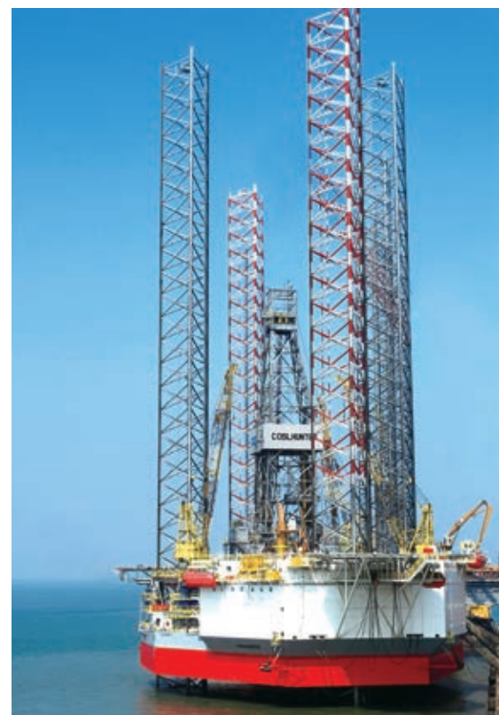
CJ-46 series of self-elevating offshore drilling rig built by China Merchants Industry
